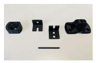
Although the 3D printed components have a shorter lifespan than the original metal jaw, the cost-benefits of using Additive outweigh the original part function.
