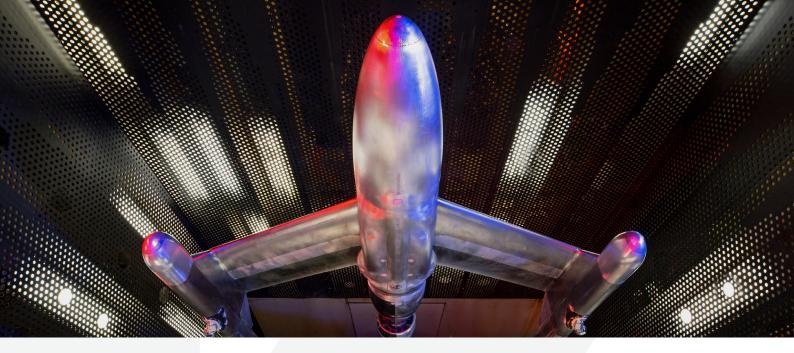
**Shape definition to manufactured component** The nose cone was made from aluminium 2319 wire feedstock. The near-net shape was produced in WAAM3D's large format 3D metal additive printing platform - RoboWAAM<sup>®</sup> and was carefully monitored throughout the deposition process by ARA and WAAM3D.
