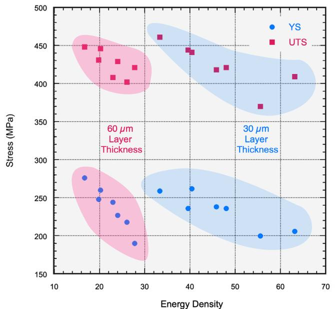
**Figure 5:** Plot of yield strength and UTS as a function of energy density for the 14 different parameter combinations that were explored.
