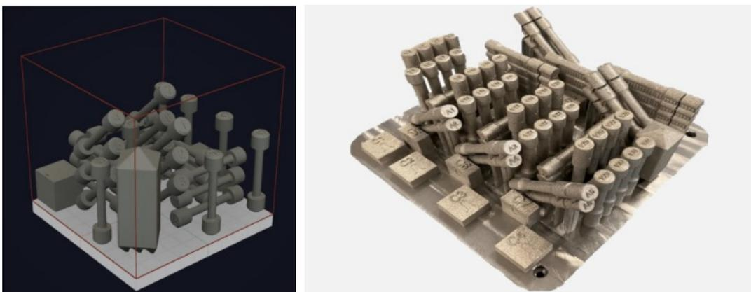
**Figure 1:** Example qualification builds for (a) an XACT metal 200C and (b) a Renishaw 500Q
