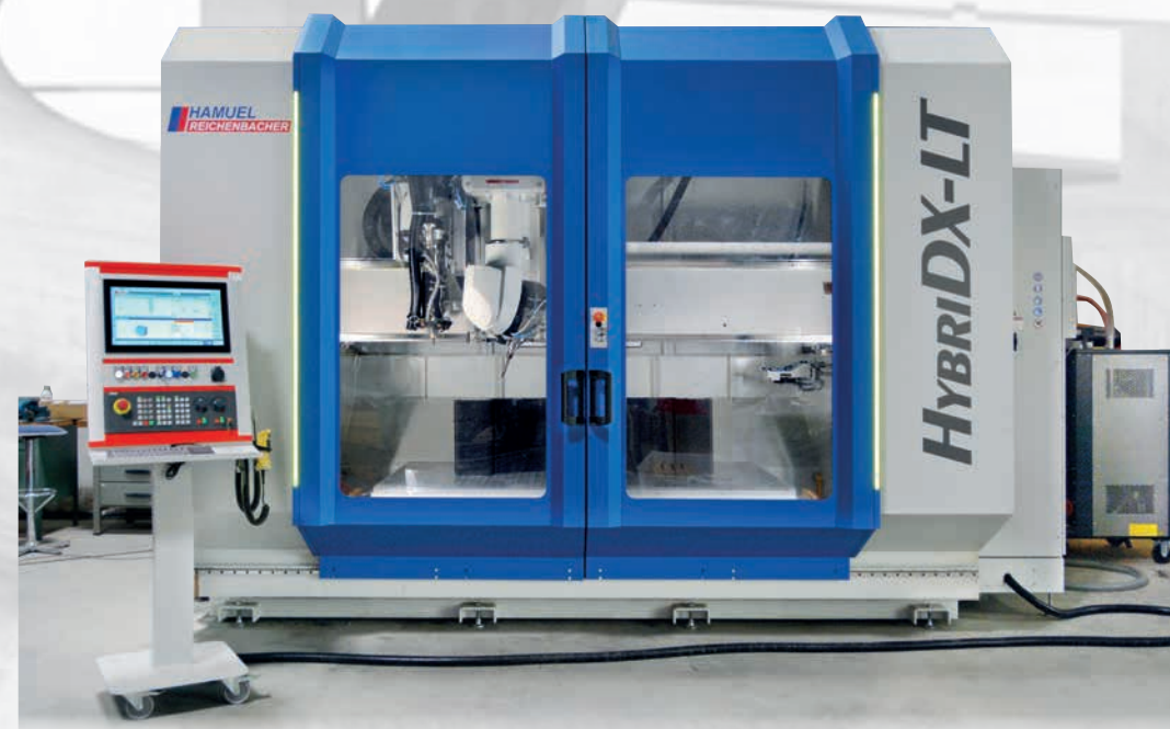
CNC machining centre HybridDX-LT for additive and subtractive manufacturing.
