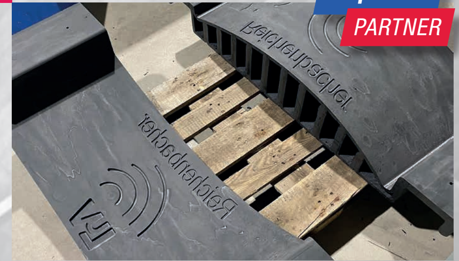
Concave and convex form part with a milled-in individual surface structure.
