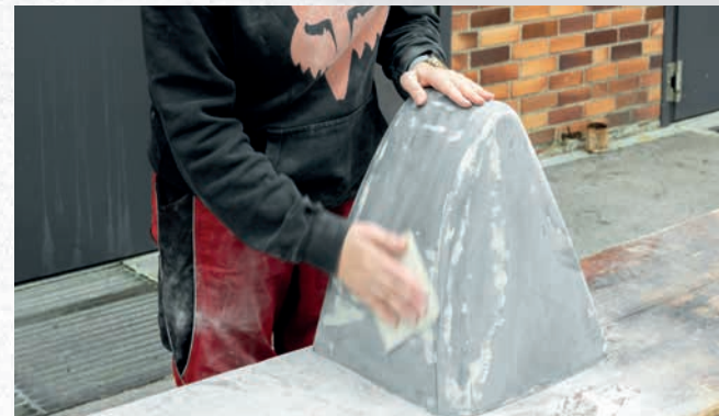
The CAT-Racing team further processed the deep-drawn parts, among other things carrying out grinding work to refine the surfaces.
