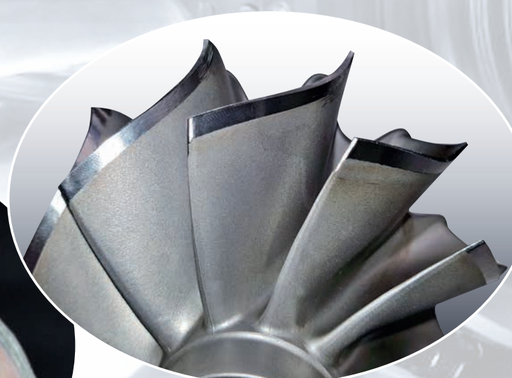
Repaired compressor wheel.
