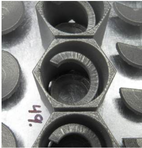
Close up: Support-free spiral helix with 20° overhangs
