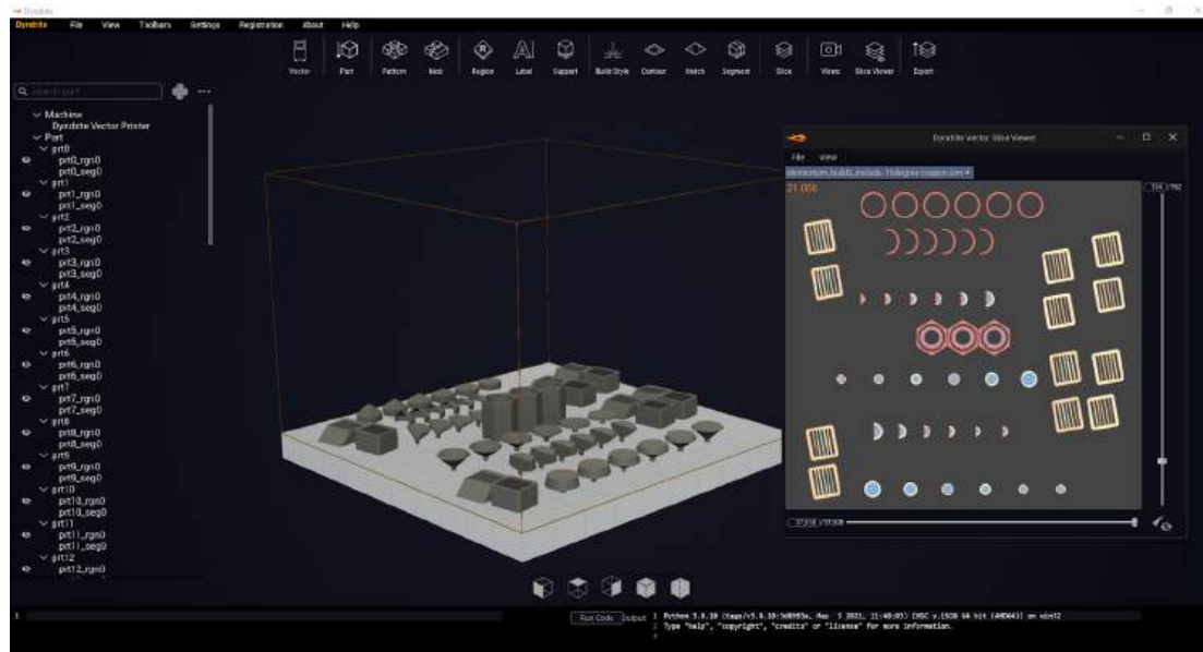
Figure 2a: Dyndrite LPBF Pro screenshot of build plate and slice viewer featuring range of geometry types, including overhangs, thin walls, slanted thin walls, and spiral helices
