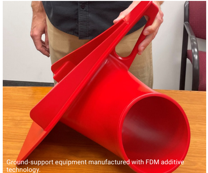
An aircraft duct 3D printed with ULTEM™ 9085 resin material.
