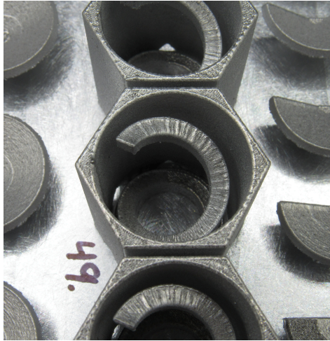
Close up: Support-free spiral helix with 20° overhangs
